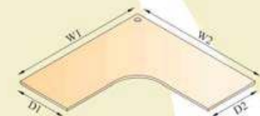
CURVILINEAR TOP (TYPE-3) W1=1200,1350,1500,1650,1800 W2=1200,1350,1500,1650,1800 D1=450,500,600,750 D2=450,500,600,750
